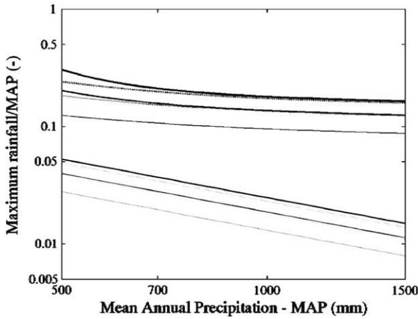
Fig. 3. Example of relationship between MAP and  $\eta_{t,T}$  for  $t = 15$  min (grey lines) and 24 h (black lines),  $T = 10, 100$  and 1000 years (thin, medium and thick lines, respectively), and EV1 (dashed lines) and GEV (solid lines) parent distributions.
