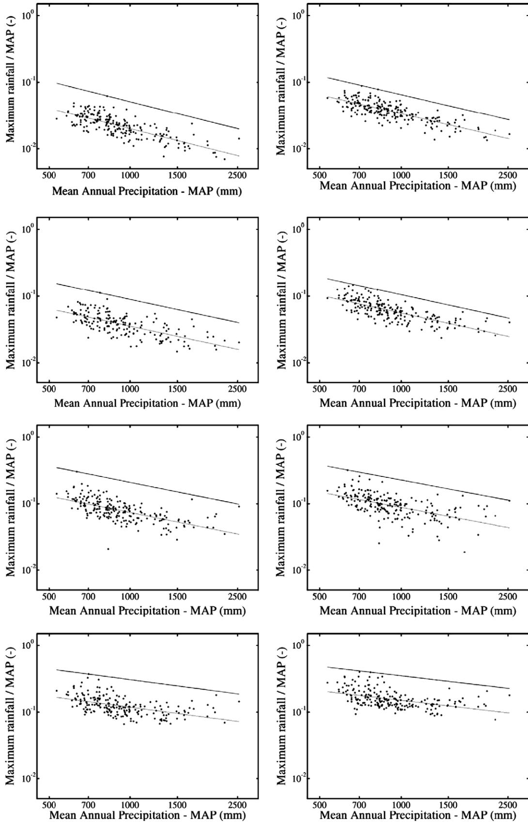
**Fig. 8.** DDEC (thick lines) constructed for the study area for duration (from top to bottom and from left to right): 15, 30 and 45 min and 1, 3, 6, 12 and 24 h (right), each diagram reports also the observed rainfall maxima (dots) and the regression line between maxima and MAP (thin line).
