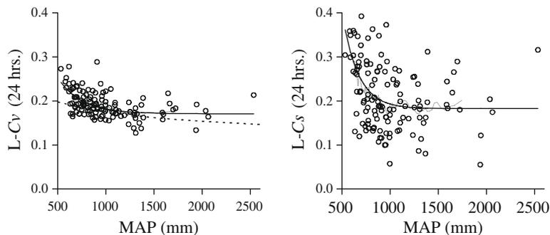
Fig. 1. AMS of 24 h rainfall for a large region in northern-central Italy: sample  $L$  moments vs. MAP (circles); weighted moving average curves (gray thick line); relationships between  $L-Cv$  and  $L-Cs$  and MAP identified by Di Baldassarre et al. (2006) (solid black line) and between  $L-Cv$  and MAP identified for Canada by Alila (1999, Table 3, p. 650) (dashed black line).
